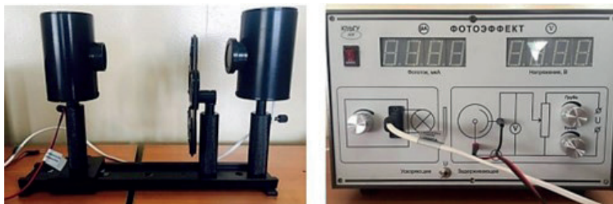
Figure 1. Optical bench and electronic unit for studying the photoelectric effect
