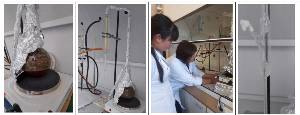
Figure 2 – Extraction of essential oil in the Clevenger apparatus
