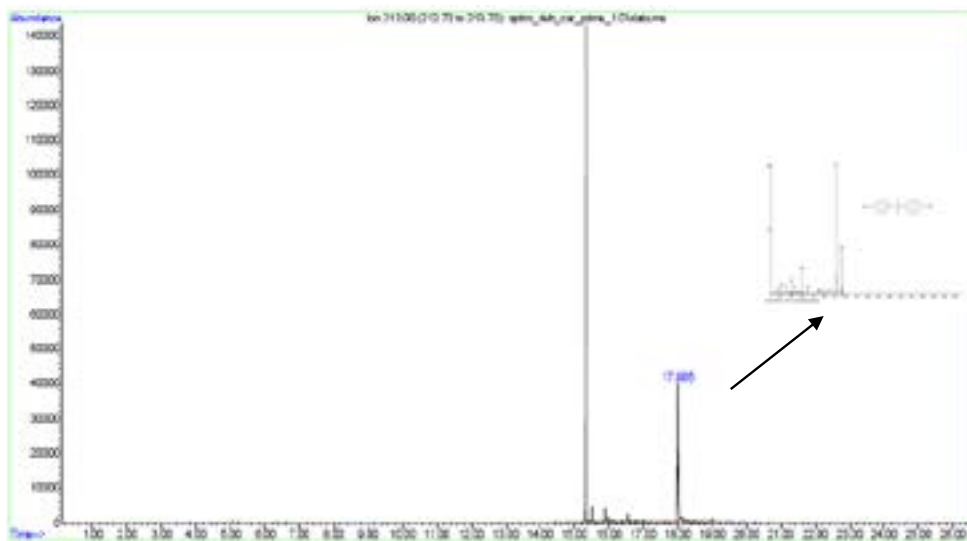
Fig. 2. Chromatogram and mass spectra of bisphenol-A
