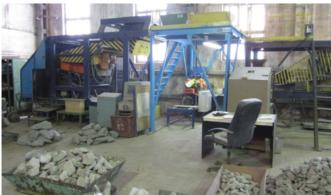
Figure 4 - Experimental-industrial sector with separators SRF2-300 and SRF1-100
