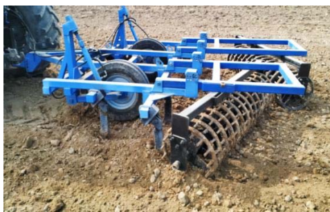
Figure 4 – Experimental combined machine with a ring-bar roller
