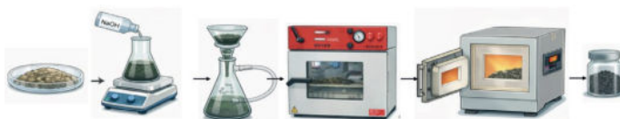
Figure 3. Scheme of the procedure to obtain the MnFe 2 O 4 /Shymkent reference clay.
