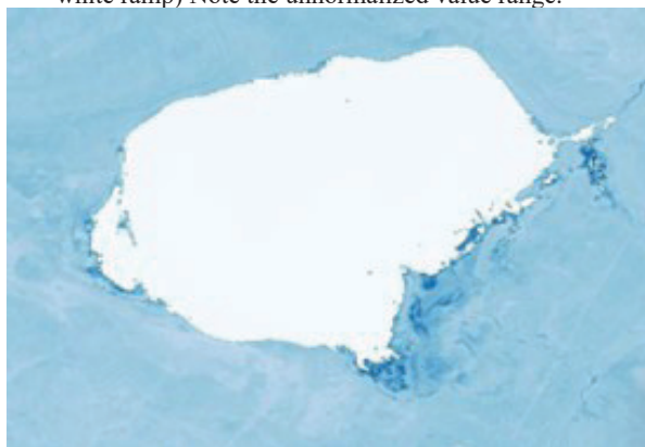
2-Figure. NDWI map of Lake Akkol generated in Python using pseudocolor rendering (blue to white ramp) Note the unnormalized value range.
