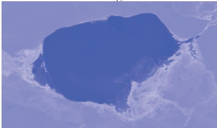
3-Figure. NDWI map of Lake Akkol generated in GEE using pseudocolor rendering (blue to white ramp)
