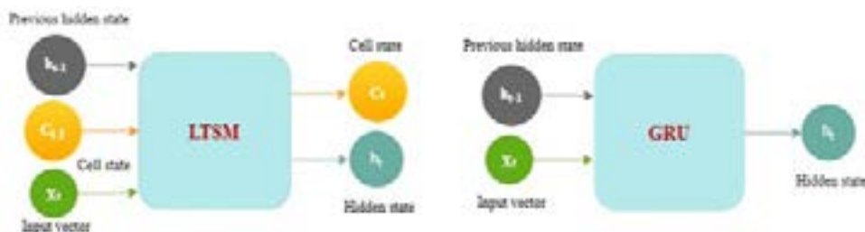
Fig. 2. LSTM and GRU architectures
