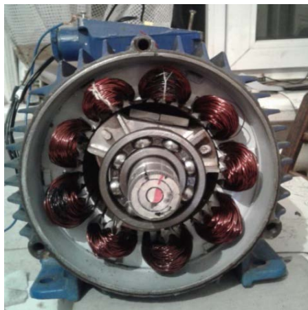
Figure 3 Photo – Symmetrically wound 9 stator windings
