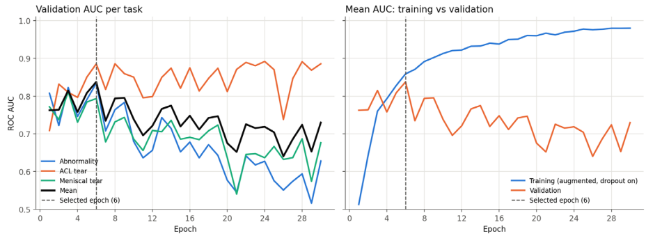
Figure 5 — Left: validation AUC per task and their mean for the multi-task run. Right: training mean AUC (with augmentation and dropout active) against validation mean AUC. The dashed line marks the selected epoch (6).
