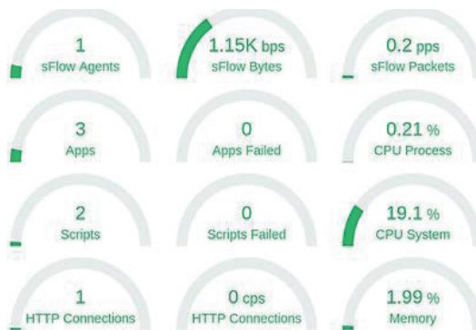
Figure 13 – sFlow Image During Ping Test to Network Users
