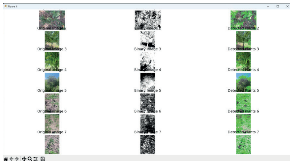
Fig. 10 – Photos of plants in the field (original image, binary image, detected plants)
