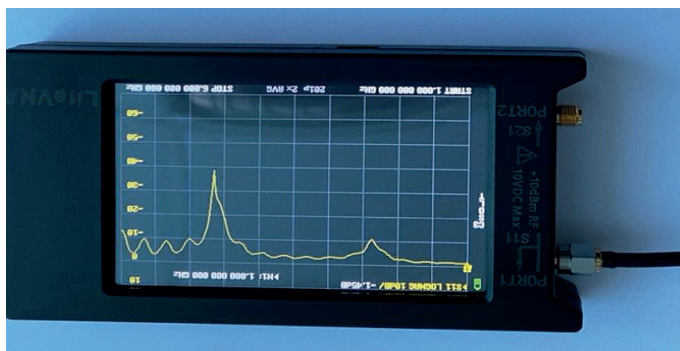
Figure 3 - Fabricated wearable Yagi-Uda antenna result at Nano VNA analyzer
