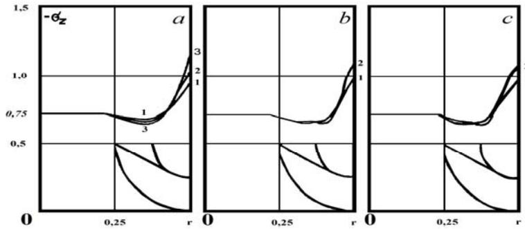
Figure 2(a, b, c) - distribution of the contact stresses  $-\sigma_z$  resulting from point-in-time  $t = 0,25$
