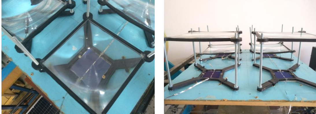
Figure 3. Laboratory layout of a concentrating solar cell
