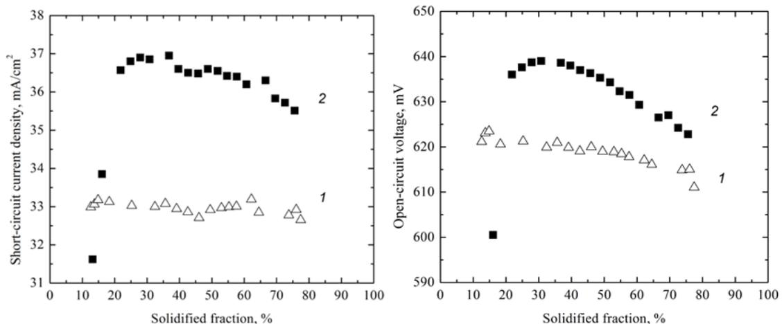
Figure 5 - Comparison of changes in  $V_{\text{oc}}$  (left) and  $J_{\text{sc}}$  (right) along the height of ingots for solar cells made of ML-Si and mc-Si: 1 - mc-Si, 2 - ML-Si
