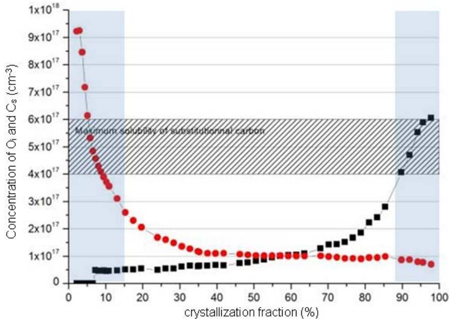
Figure 2 - The concentration of O<sub>i</sub> (points) and C<sub>s</sub> (squares) obtained by IFTS measurements along the ingot height. The shaded rectangles highlight the cut off areas on the top and bottom of the ingot, the shaded area shows the maximum solubility of C<sub>s</sub> in silicon
