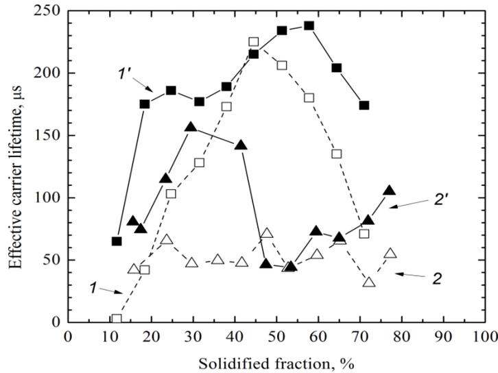
Figure 4 - Comparison of the effective lifetime (with an excessive concentration of charge carriers,  $\Delta n = 1 \cdot 10^{15} \text{ cm}^{-3}$ ) on the ML-Si wafers of the central brick and mc-Si, depending on the height of the ingot:
