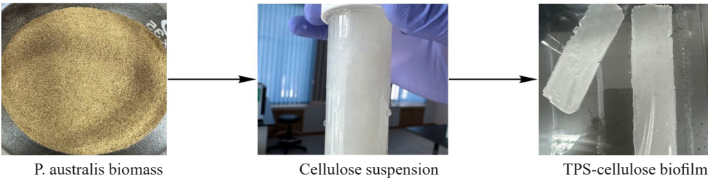
Figure 1 — Preparation process of TPS-cellulose biofilm from Phragmites australis biomass.
