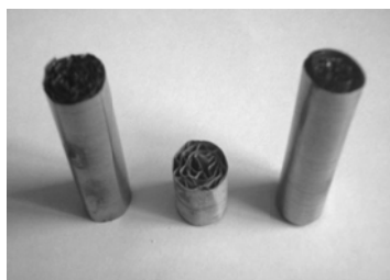
Figure 1- The samples of catalysts on metal blocks for laboratory tests
