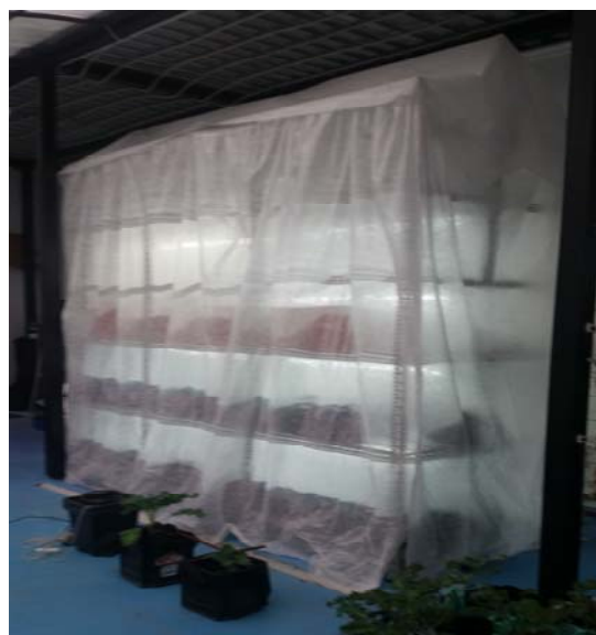
Left - case for regulating gas lifted for servicing, right - cover protects shelving, creating an optimum microclimate for plants. Photo 5 - Hothouse shelf during in vitro cultivation experiments
