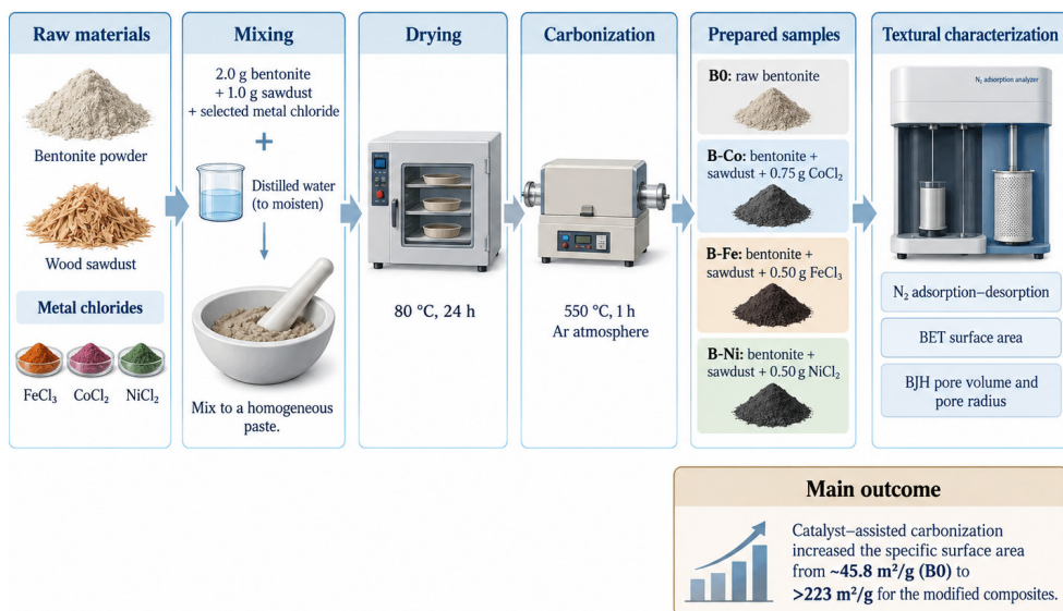
Figure 1 — Preparation and textural characterization route for the bentonite–sawdust composites. Note: compiled by the authors from the experimental procedure used for the analyzed samples.
