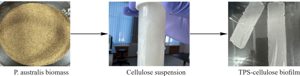
Figure 1 — Preparation process of TPS-cellulose biofilm from Phragmites australis biomass.
