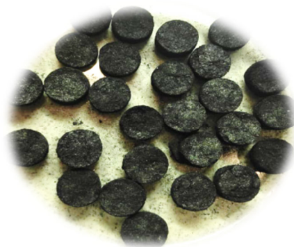
Figure 2 – Rice husk oil sludge: activated carbon obtained in the ratio of lignosulfonate 9: 1: 2.
