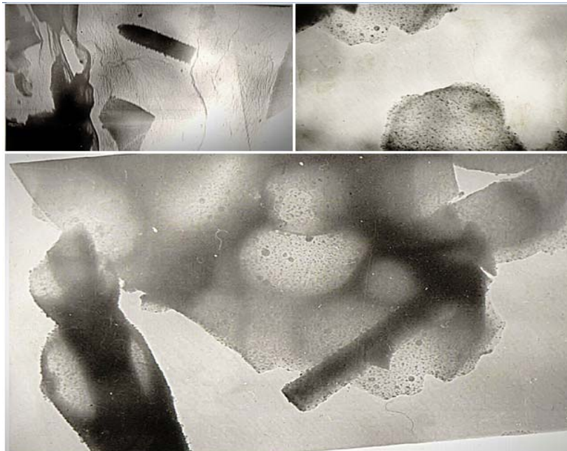
Figure 1 - TEM images of the 50 % Ni - 50 % Al – (0.05%)Pt- glycine catalyst before tests
