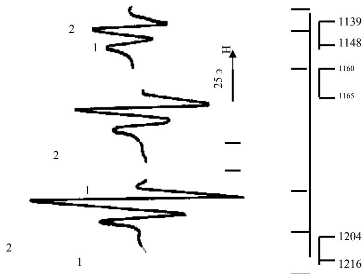
Figure 1- Change of EPR signal of oils in the section of the Kotyrtas North field, well 23.
