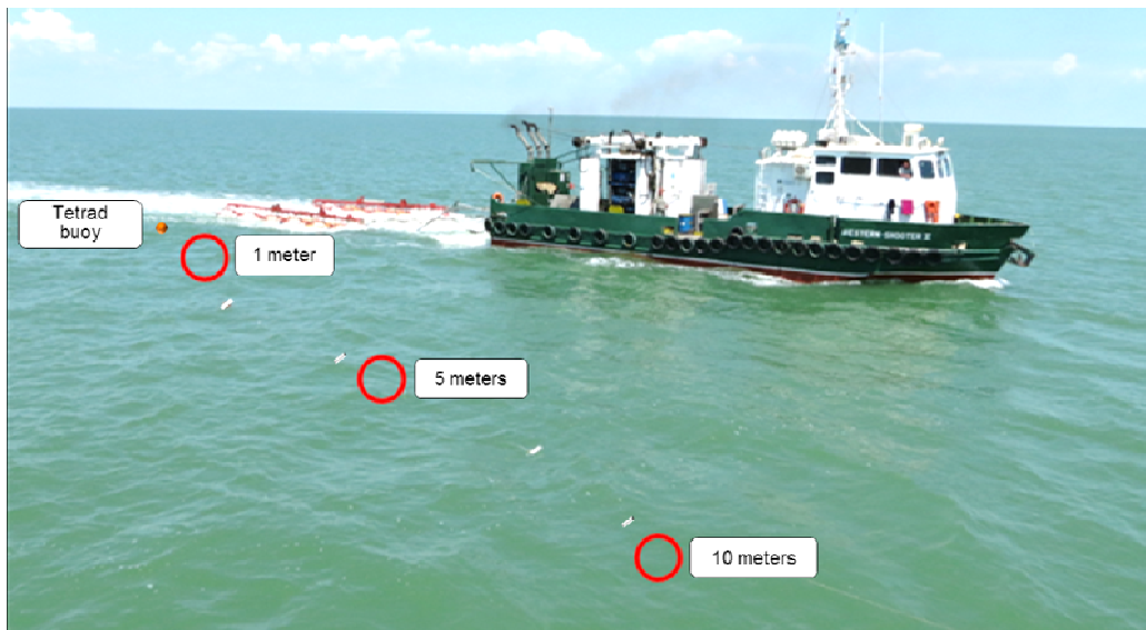
Figure 2. Scheme of the location of stations to study the impact of seismoacoustics on aquatic organisms
