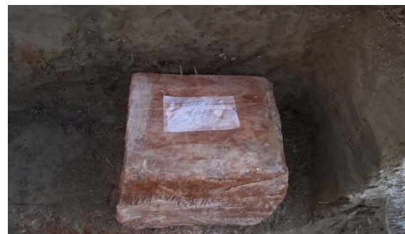
Figure 4 - The resulting monolith of undisturbed structure
